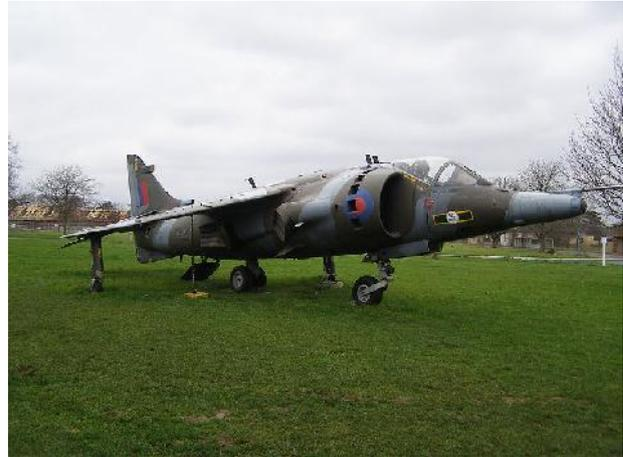
The Hawker Siddeley Harrier GR.1/GR.3 and the AV-8A Harrier are the first generation of the Harrier series, the first operational close-support and reconnaissance fighter aircraft with Vertical/Short Takeoff and Landing (V/STOL) capabilities, colloquially referred to as a "jump jet". The Harrier was the only truly successful V/STOL design of the many that arose from the 1960s.
